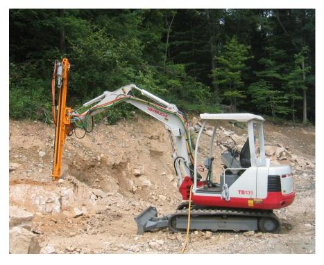
Turns any Mini Excavator into a Powerful and Productive Rock Drill in Minutes
